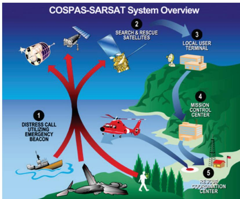
There are two types of 406 EPIRBs which are activated in different ways. Automatically if your boat sinks (Category 1, float free, automatically activated), or Manually by you (Category II). Once activated in an emergency situation the EPIRB should remain in the 'on' position.
